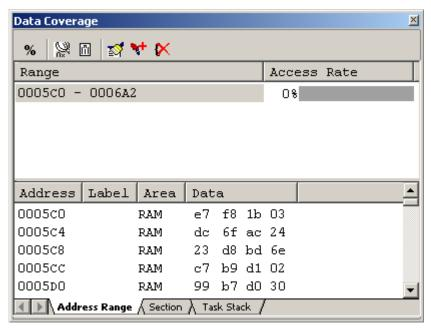
Figure 5.107 Data Coverage window (address specification)
